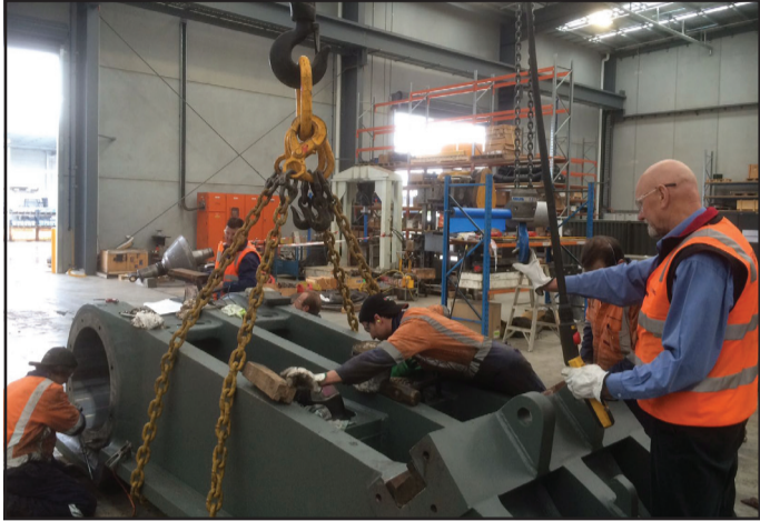
Photo 1 Terex Jaques rebuilding jaw crusher
